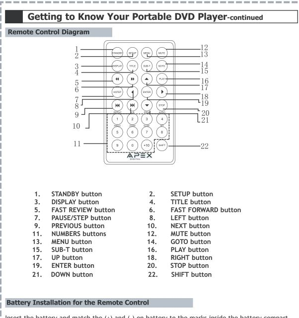
Insert the battery and match the (+) and (-) on battery to the marks inside the battery compartment.
